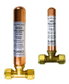
The SURGEx-COMP series offers piston-operated, lead-free water hammer arrestors made from hard-drawn seamless copper with a brass compression TEE, available in size DN15 (½"). These arrestors absorb shock caused by sudden changes in water flow direction to prevent damage to pipes, valves, and fixtures. These arresters are usually used in copper tubes.
