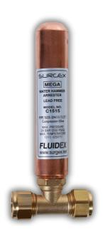
The SURGEx-COMP series provides piston-operated, lead-free water hammer arresters constructed with hard-drawn, seamless copper and brass compression TEE. These arresters, available in size DN15 ( $\frac{1}{2}$ "), can absorb the shock caused by sudden changes in water flow direction, thereby preventing damage to pipes, valves, and fixtures. Typically, these arrestors are compatible with copper piping.
