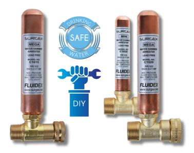
The SURGEx-DIY series offers piston-operated, lead-free water hammer arrestors made from hard-drawn seamless copper with a brass TEE, available in sizes DN20 (3/4") and DN15 (1/2"). These arrestors absorb shock caused by sudden changes in water flow direction to prevent damage to pipes, valves, and fixtures. They are suitable for use in washing machines, dishwashers, and general plumbing applications.
