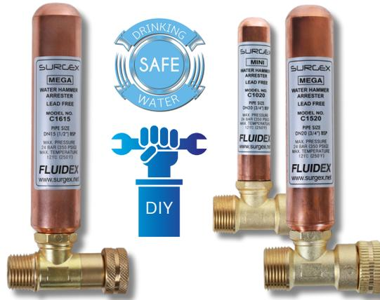
The SURGEEx-DIY series offers piston-operated, lead-free water hammer arrestors made from hard-drawn seamless copper with a brass TEE, available in sizes DN20 (3/4") and DN15 (1/2"). These arrestors absorb shock caused by sudden changes in water flow direction to prevent damage to pipes, valves, and fixtures. They are suitable for use in washing machines, dishwashers, and general plumbing applications.
