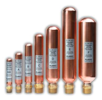
SURGEx-LFC series is a piston operated, water hammer arrester fabricated from hard drawn seamless copper with NPT or BSP threaded male LEAD-FREE brass end connections. SURGEx LFC arresters are available in sizes AA thru F and have connection diameters from 1/2" to 1".
