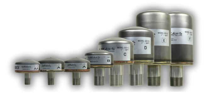
The SURGEx-S series is a pre-charged, all stainless steel, bellows type water hammer arrester that provides excellent surge pressure absorption. SURGEx-S arrester is available in sizes AA through F with end connection ranging from 1/2" to 1". The SURGEx-S has a hermetically sealed air cushion that eliminates air loss, ensuring consistent performance. The unit is fabricated from high-grade stainless steel to withstand chemical degradation and attack from waterborne contaminants.
